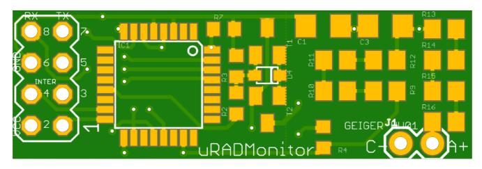
There are two connectors that you will use. Connector one, an eight pin 2x4 header connector with male pins and Connector two, going directly to the Geiger tube which is a 2 pin header connector with male pins.
