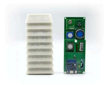
uRADMonitor® A4 is a fixed, automatic monitoring station that tracks 11 important environmental parameters, mainly various toxic gases that can impact human health. It comes in a rugged ASA/RESIN plastic housing with brackets for easy wall or pole mounting.
