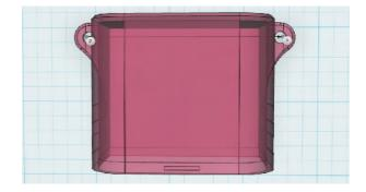
Dimensions 43 (width without ears) x 40 (height) x 27 (thickness) Distance between the centers of the holes 53mm.
