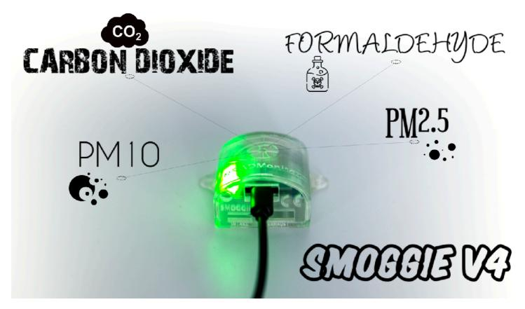
The 4th SMOGGIE comes in a transparent resin enclosure and adds LEDs to indicate the pollution level! At a glance you can see if the unit shows green, yellow or red, corresponding to real time CO<sub>2</sub> levels. The form factor remains the same so this is still world's smallest automated IOT air quality monitor.
