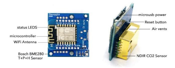
uRADMonitor SMOGGIE assembled circuit board diagram in hardware version 3
