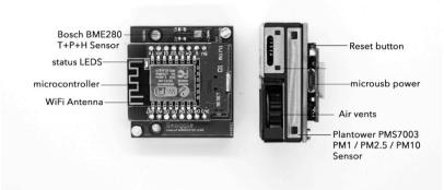
uRADMonitor SMOGGIE is an automated, fixed monitoring station. There are 4 SMOGGIE flavors for different applications. They all track temperature, pressure and humidity. Additional features include:
