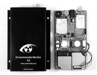
uRADMonitor A3 is an automated, fixed monitoring station that tracks a total of 9 important air quality parameters. It comes in a compact, rugged aluminum enclosure with wall mounting support. The data is exported to the uRADMonitor network and can be accessed in real time using the cloud API interface or directly via the local network. Four variants are available with the same sensors but different connectivity options: Ethernet, Wifi, GSM/Cellular and LoRAWAN.
