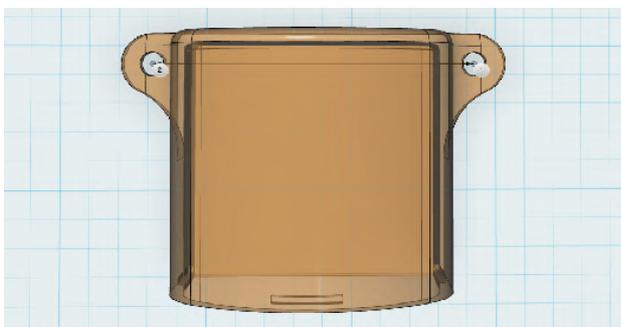
Dimensions 43 (width without ears) x 40 (height) x 27 (thickness)
