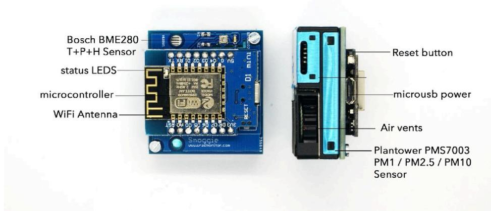
uRADMonitor SMOGGIE assembled circuit board diagram in hardware version 1
