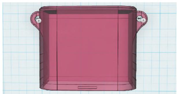
Dimensions 54 (width without ears) x 44 (height) x 35 (thickness)
