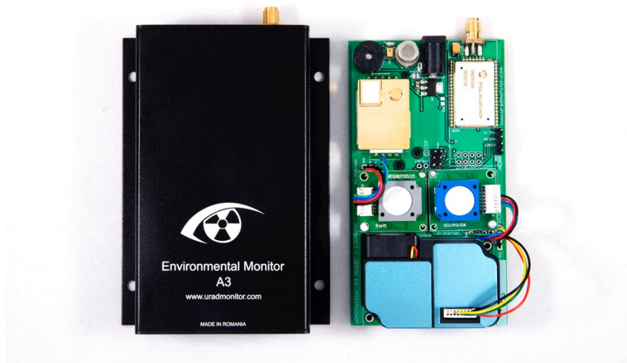
Fig. 1 uRADMonitor A3, fixed air quality monitoring station
