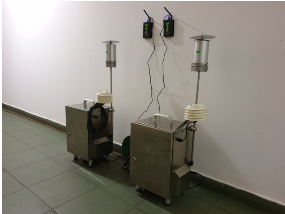
Fig. 2 uRADMonitor A3 units and the sampling units Sven Leckel LVS3.
