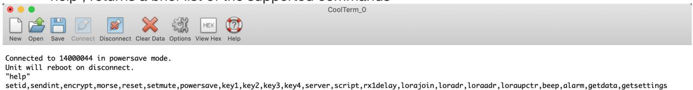
Figure 6. Device response to the help command, showing the list of supported commands
