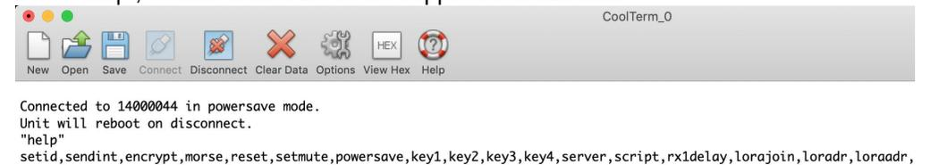
Figure 12. Device response to the help command, showing the list of supported commands
